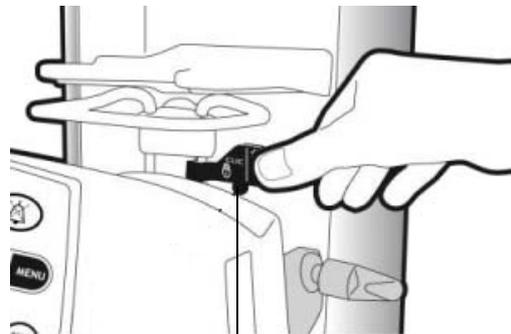
Pump release mechanism lever
