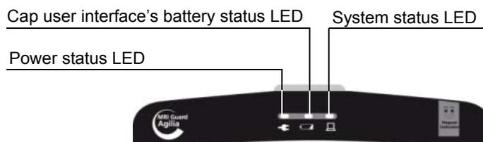
The **MRI Guard Agilia** provides the user with visual information about the power supply, the cap user interface's battery and the system status indicated by a specific display located at the top of the device.
