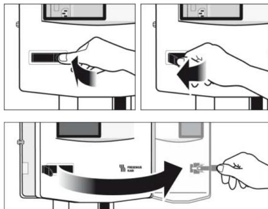
2. Ensure the pole clamp of the pump is folded up against the pump. Position the **Agilia** IV infusion pump in front of the **Link+ Agilia** and slide it carefully on the pump shelf slot.
