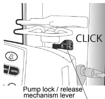
4. Pull the pump out to check if well installed.
